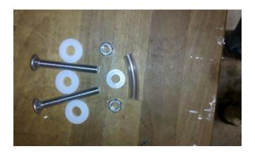
The white washers are 1/4" UHMW Polyethylene. Made these too! 3/8" Stainless Steel carriage bolts, washers, and nuts. The clear tube slides over the bolt, which helps the chair collapse without harm (1/2" holes in the wood).
