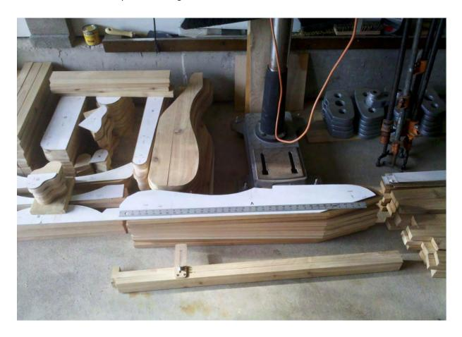
Most of the pieces had to be "paired" for grain and matching hole location. Then identified as part of Chair 1, 2, 3, and 4 early in the process. Sharpie to the rescue! It took about a week to drill all of the necessary holes. Below are the Forstner bits required and the Stain [Sikkens Cetol 1, Dark Oak].
